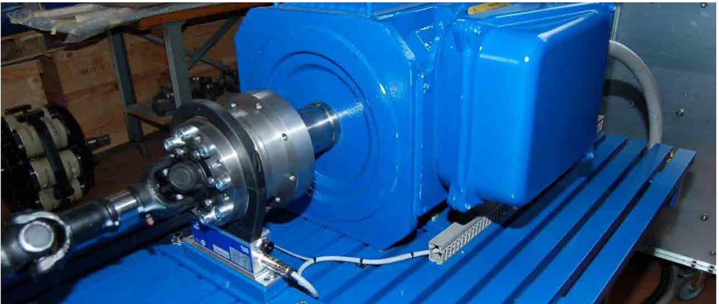
In order to develop a test bench for electric car engines, Dynosens needed an interface to connect its T40B torque transducer to the EtherCAT fieldbus. The TIM-EC that HBM was in the process of launching was put to operational use straightaway ...
