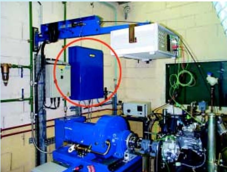
DMC 202 with its protection cover, installed in a test cell
