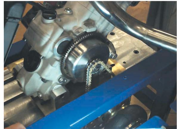
With the increase of engines using a left hand output, DynaKart has been designed to take this change into account. Mounting and removal of the engine and quick changes of transmission ratio are made easy with the universal mounting bracket.
