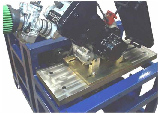
The brake is mounted in balance and its rotation is reacted against by a sensor which, measures the brake torque. This is directly comparable with the transmitted torque in the transmission shaft of a kart. With Eddy current technology, the brake is extremely precise and has an excellent response time. It is cooled by 'channelled' air flows in which cold and warm air is separated. This allows increased brake capacity and longer running times.
