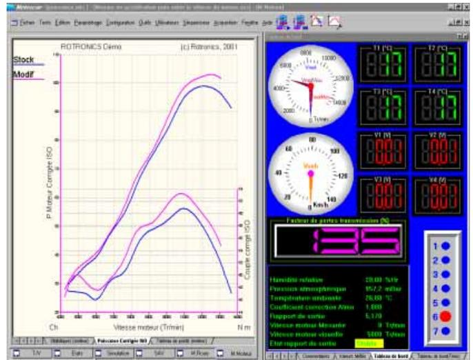
Ignition defect in a four cylinder engine, the curve indicates a loss of power at 112 mph or approximately 7000 rpm. Thanks to the engine speed kit, an ignition anomaly is identified (transient problem in cylinder 3).
