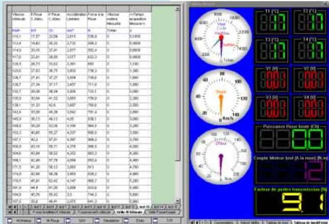
Table of power development and acceleration for this two-cylinder two-stroke. Also available in a graphical format, this diagram allows the identification of possible losses of traction. The power at the wheel depending upon the chosen gear, in the case of "wheel spin", the test will be carried out in a higher gear in order to limit the stresses applied to the tyre.
