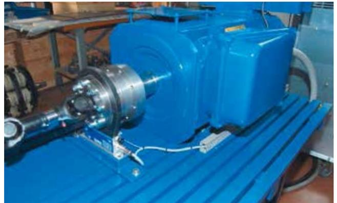
The motor test bench developed by Dynosens for electric vehicles, with T40B torque transducer and TIM-EC EtherCAT interface module
