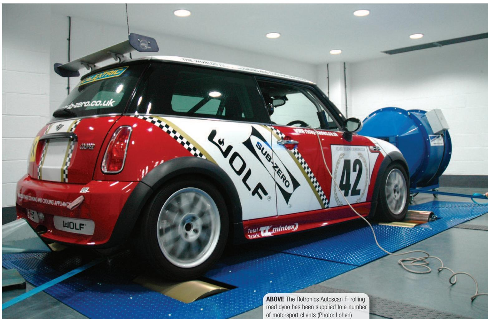
**ABOVE** The Rotronics Autoscan Fi rolling road dyno has been supplied to a number of motorsport clients (Photo: Lohen)
