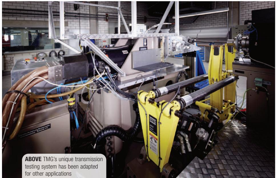
ABOVE TMG's unique transmission testing system has been adapted for other applications
